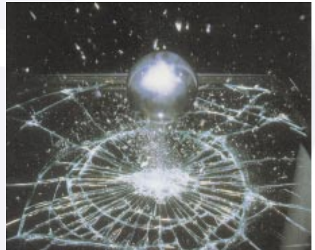
Madico Protekt clear safety film undergoing steel ball impact test
